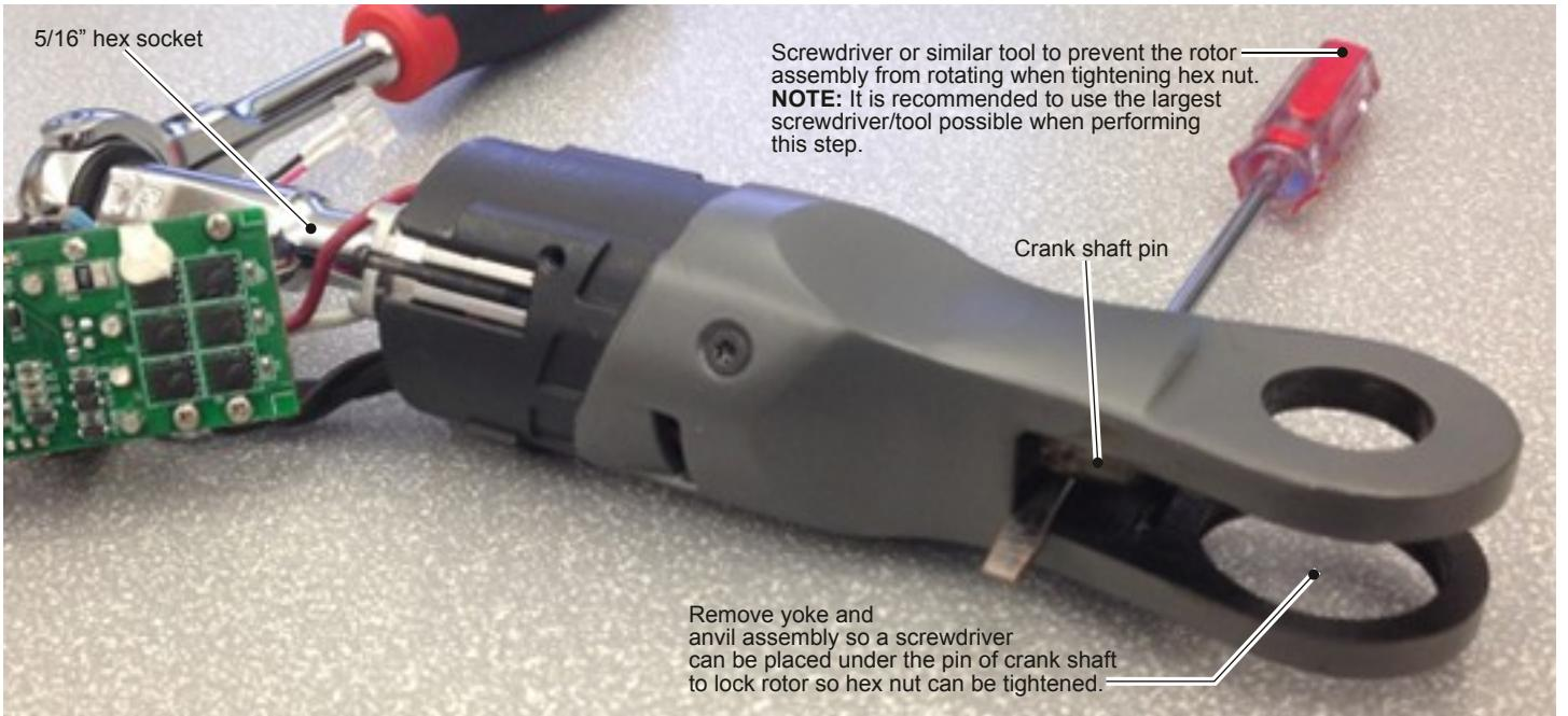
To properly tighten hex nut (20) to rotor (33), it is important to lock rotor and keep it from spinning. The recommended approach is illustrated above.
